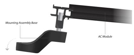
If adjustments need to be made to one or both of the mounting assemblies in row two, turn the *Mounting Assembly Base* in either direction to adjust its height. To raise the height, turn the base clockwise. To lower the height, turn the base counterclockwise.
