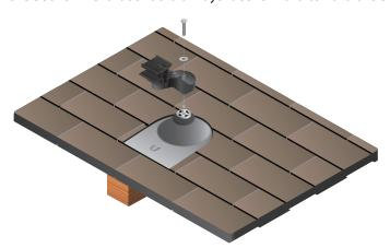
2. The mounting base and swivel portion for each mounting assembly should be facing towards the front as shown. (Note: You may need to adjust the position of the mounting assemblies as you proceed, so you can leave the mounting bolts slightly loose for the time being.)
