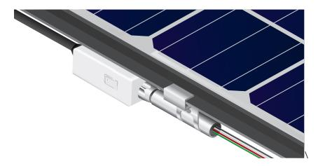
10. On the opposite end of the string of *AC Modules*, terminate the open Y-Cable connector using the cable end cap.
