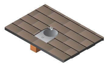
16. Apply a minimum of 1/4" (6 mm) continuous roof caulking around the gap between the flashing and roof mount.
