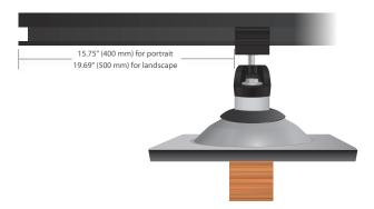
5. Once the first roof mount location is marked, continue to mark additional roof mount locations along each horizontal chalk line observing the maximum mount spacing for your location until the desired array layout is complete. Check the opposite end of the array to ensure the cantilever distance has not been exceeded at any other locations in your array.
