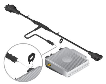
3. Connect the AC trunk cable (that was previously connected to the Microinverter) to the *Output* connector on the Solar Gateway.
