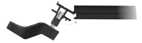
3. While lowering the *AC Module* into place, continue to pull the top edge of the solar panel slightly towards you to ensure it remains hooked onto the swivel mounts in the previous row. Secure the *AC Module* to the *Roof Mounts* using the mounting hardware. If the *AC Module* is not seated properly or sitting evenly with the mounting hardware in row one, make the necessary adjustments.
