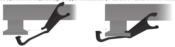
Cables then snap into the *Cable Clip* underneath the *AC Module*, holding them in place along the inside edge of the *AC Module*'s frame.
