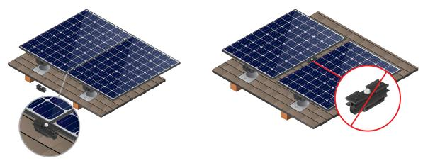
When you have multiple mounts on a *Solar Panel* or one right next to a connector, do not install the mount closest to the connector. Leave it loose temporarily, allowing the *Solar Panel* to drop quite a bit where they come together and make it easier to level the array panels.
