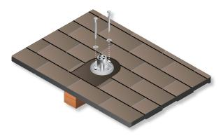
12. Slide a prybar under the roof shingles where the flashing is to be installed to break the bond between the roof courses. Remove any nails from shingles that will interfere with the flashing installation and lift up the shingles.
