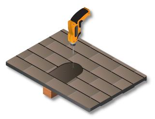
10. Cover both hole openings with roofing sealant. This will ensure watertight installation once the lag screws have secured the roof mount to the rafter.
