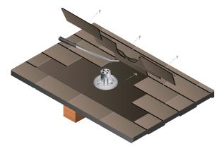
13. Apply roof sealant to the underside of the Flashing and spread evenly across the bottom surface.
