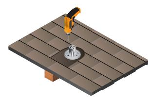
9. Remove the roof mount temporarily and finish predrilling two 3/16" (4.8 mm) holes approximately 2" (50 mm) deep.
