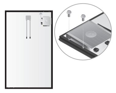
4. Connect both cables on the junction box to the DC ports on the *Microinverter*. Each cable only fits one way into its respective port on the *Microinverter*.
