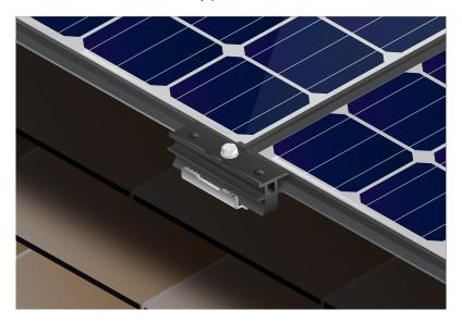
The *Panel Connectors* have preset gaps on them where the *Solar Panels* will sit as they come together. Align the gaps with the frame edges, hook them underneath, and pivot down.
