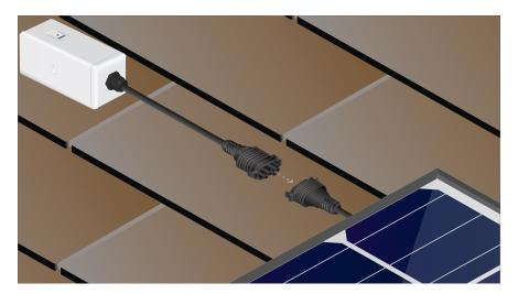
3. Thread the conduit connector into the End Run cover.
