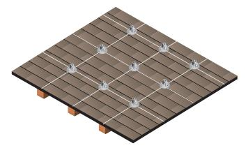
7. The roof shingles need to be cut to allow proper installation of the roof mounts and flashing. Use a chalk stick to mark a 2" (50 mm) area around the roof mount (to use as a guide) and trim the second course of shingles.
