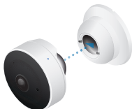
Mount Camera to Magnetic Base
