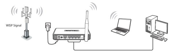
Figure 2-1 Hardware Installation of the TL-WR743ND in AP Client Router mode
