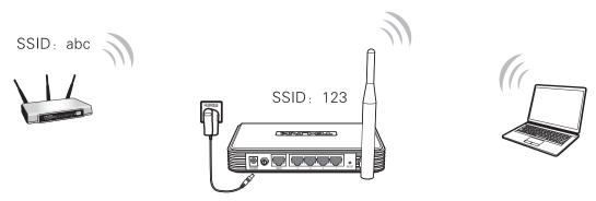
Figure 2-4 Hardware Installation of the TL-WR743ND in AP Bridge mode
