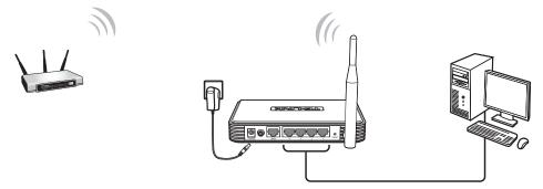
Figure 2-5 Hardware Installation of the TL-WR743ND in Client mode
