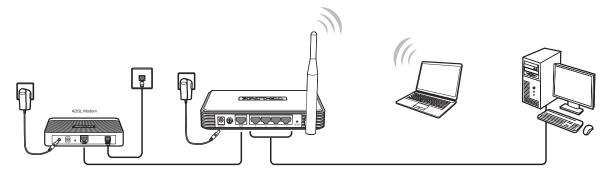
Figure 2-2 Hardware Installation of the TL-WR743ND in AP Router mode
