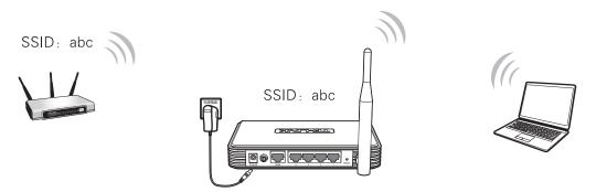
Figure 2-3 Hardware Installation of the TL-WR743ND in AP Repeater mode
