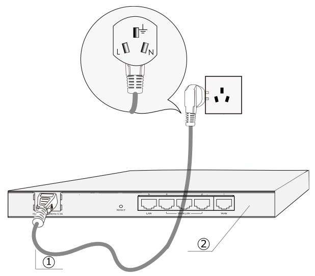
1 AC Power Cord (with PE cable) 2 Router (Rear Panel)
