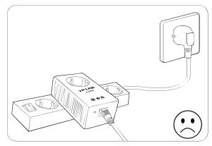
To take full advantage of the filter function of the Powerline Adapter and to improve data transmission in the network, always plug the multiple sockets into the integrated electrical socket of the Powerline Adapter.
