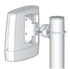
The Stationbox<sup>™</sup> can be installed on the mass, console or wall by using our NanoBracket™ Note: NanoBracket<sup>™</sup> is sold separately.
