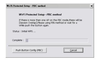
Press WPS Button on USB directly and then click the button "**Push Button Config**" shown above.
