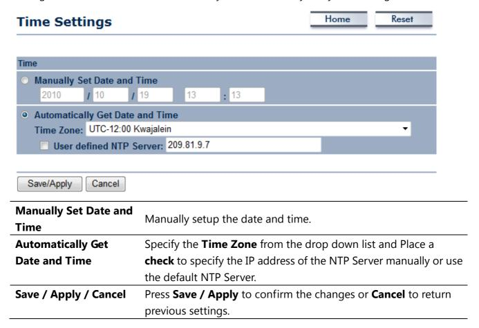
Pressing Save / Apply will change the settings immediately. It is not reversible unless the settings are changed again or the device is reset.
